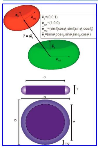
Figure 1. Scheme of the simulated objects and definitions of the geometry (see eqs 1-3 in the text). Top panel: representation of the shape of the particles and the vectors involved in the calculations. The mathematical definition of the vectors is provided in the inset. Bottom panel: Geometrical parameters of oblate spherocylindrical particles. The top and side views of a spherocylinder particle are shown.
