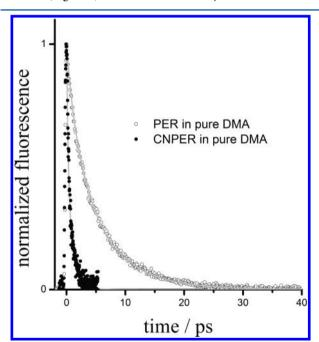
**Figure 4.** Time profiles of the fluorescence measured at 400 nm excitation of PER and CNPER in DMA. The solid lines are the calculations performed with the model.
