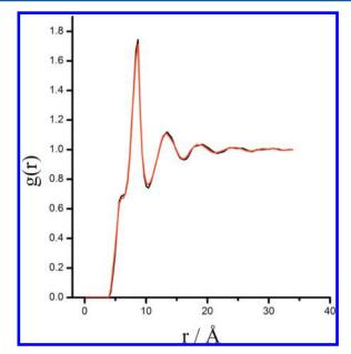
Figure 2. PER-DMA (black) and CNPER-DMA (red) radial distribution functions obtained from MC simulations.
