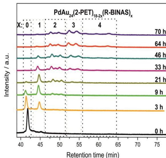
Fig. 1 HPLC chromatogram of  $\text{PdAu}_{24}(\text{2-PET})_{18-2x}(\text{R-BINAS})_x$  as a function of time. The time indicated is the time between the start of the ligand exchange reaction (addition of BINAS to the cluster solution) and injection of the reaction mixture into the HPLC system.
