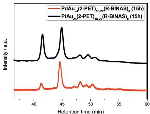
Fig. 5 HPLC chromatograms after exchange of  $\text{PdAu}_{24}(\text{2-PET})_{18-2x}(\text{R-BINAS})_x$  and  $\text{PtAu}_{24}(\text{2-PET})_{18-2x}(\text{R-BINAS})_x$ .
