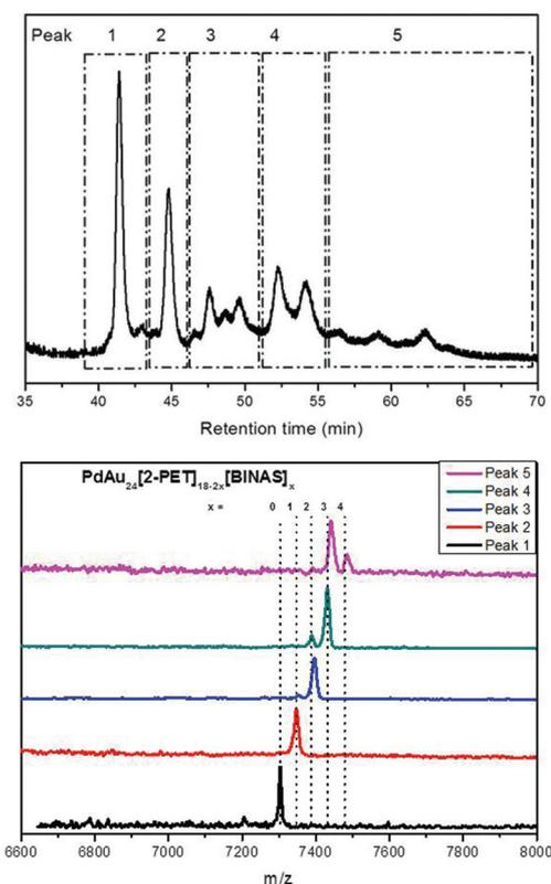
Fig. 2 HPLC chromatogram of the exchanged product (top) and MALDI-TOF mass spectra of each collected fraction (bottom). In order to obtain all species in one HPLC chromatogram, a fresh  $\text{PdAu}_{24}(\text{2-PET})_{18}$  cluster was added two times in the course of the exchange experiment. Due to slight overlapping of bands in the HPLC separation, MALDI analysis can indicate the presence of a lower exchanged product.
