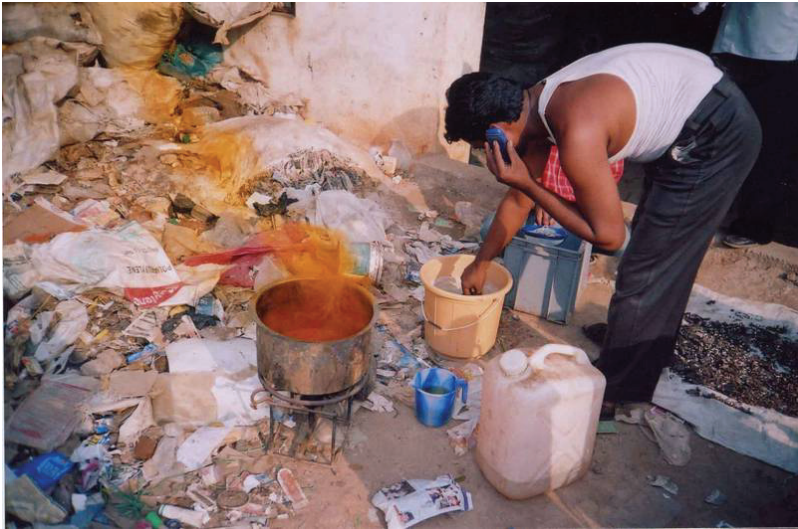
Figure 8.2: “Low –tech” gold recycling in Bangalore/India (photo by courtesy of EMPA, Switzerland)
