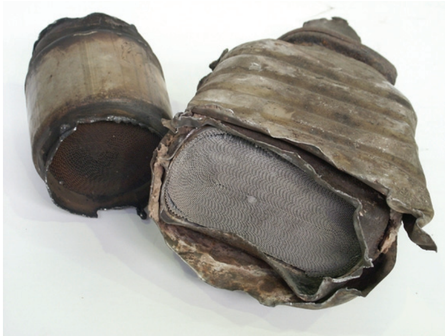
Figure 5.1: Post consumer scrap - automotive catalyst (photo by courtesy of Umicore Precious Metals Refining)
