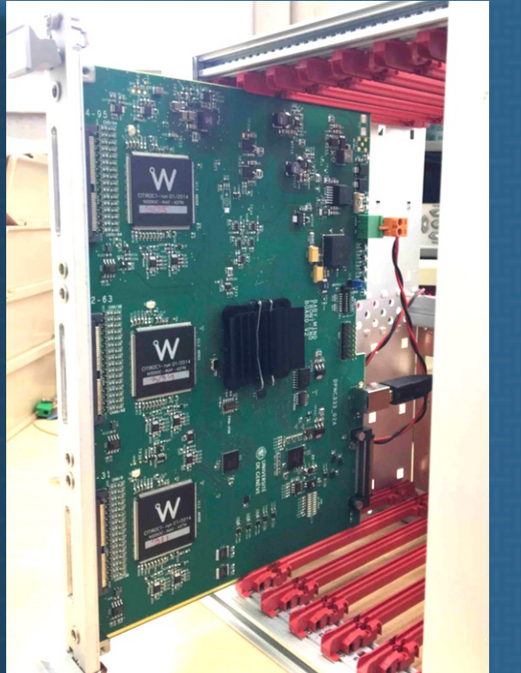
Baby MIND Front-End electronic Board (FEB).
