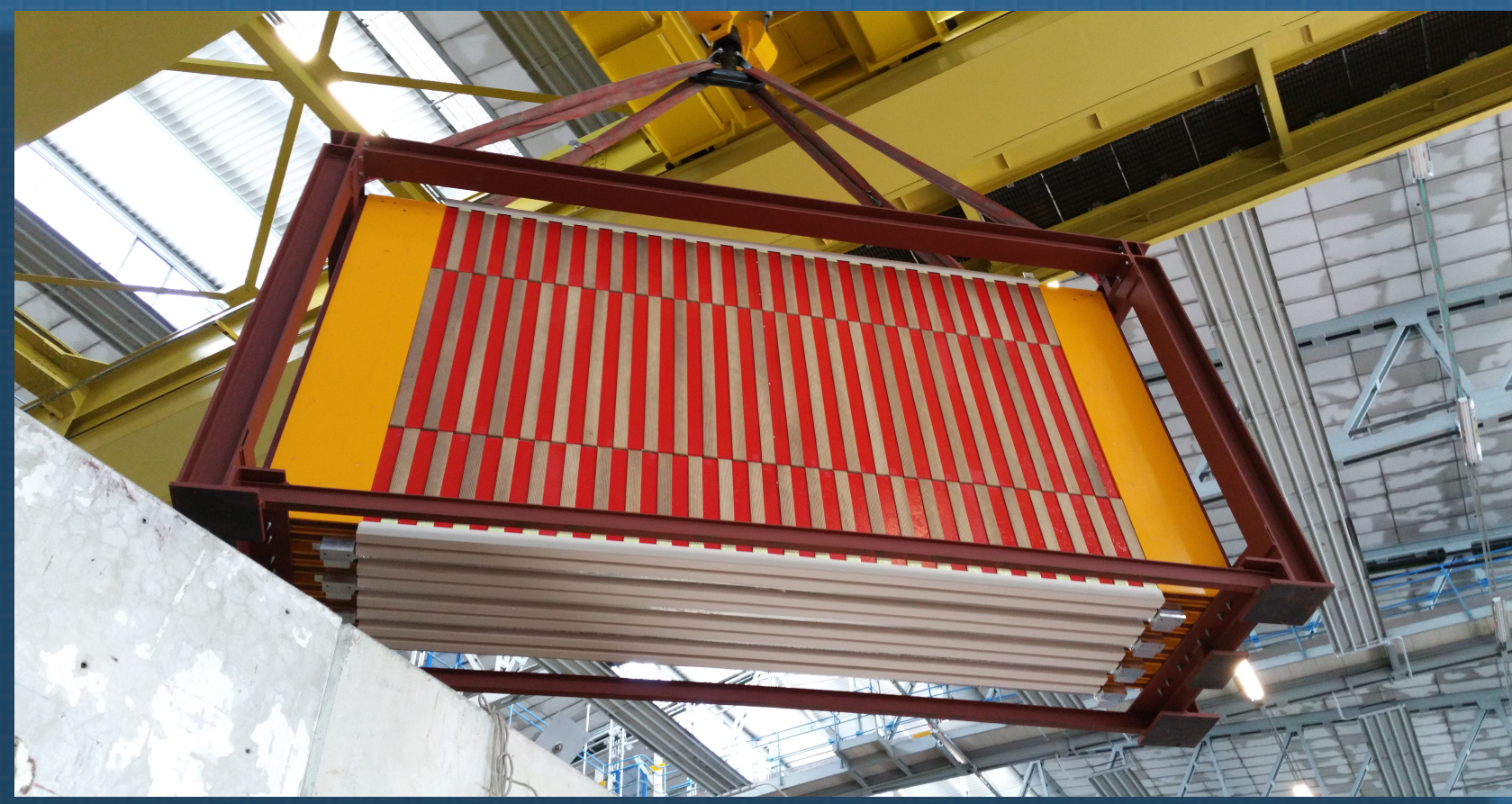
One of the four blocks of Baby MIND detector containing 8 magnetic modules and 4 scintillating modules (~20 tons).
