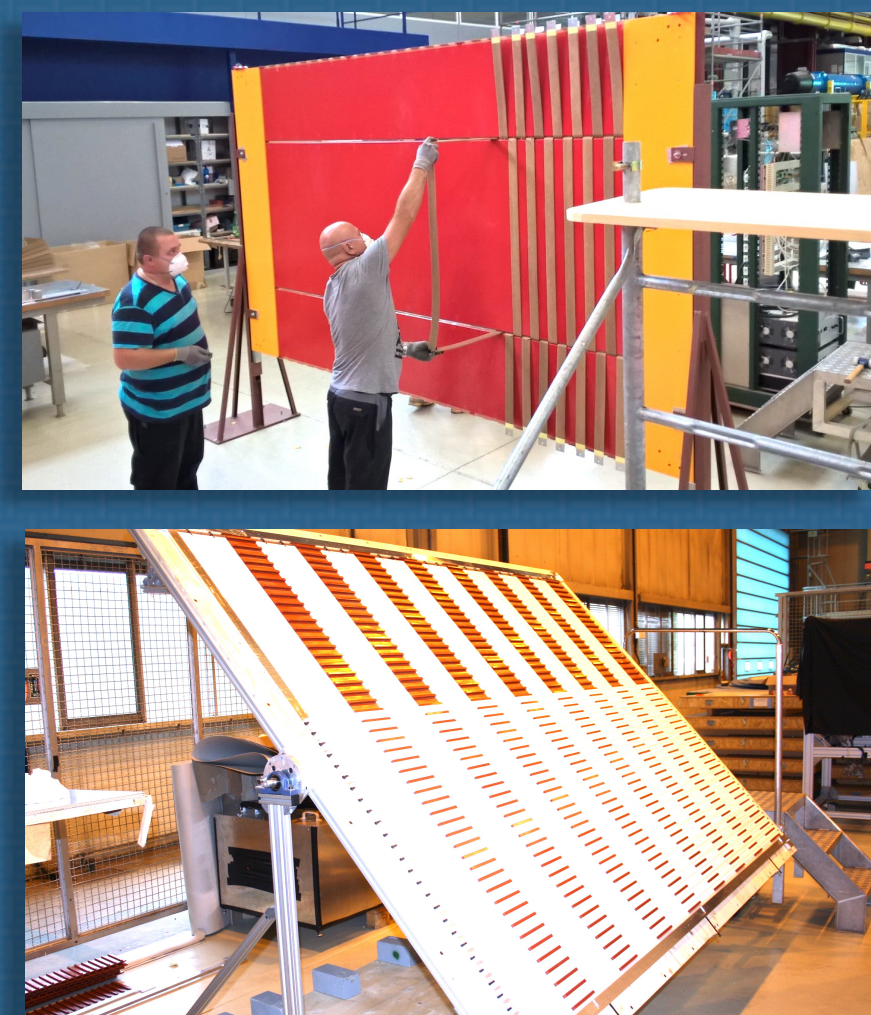
Construction of (up) magnetic module and (down) scintillating module at CERN.
