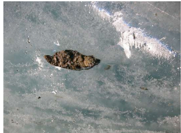
Figure 10 : Gas (mainly air) inclusions in the ice (ice tunnel) forming white bands of stratification.
