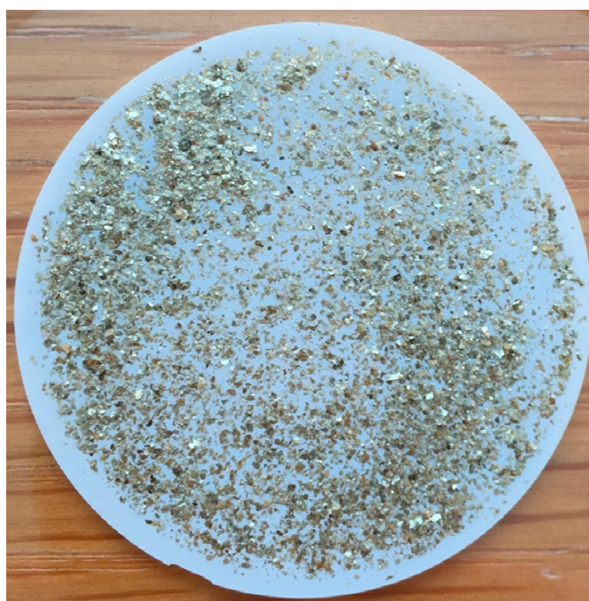
Figure 9. Buoyant particles recovered from the sample of the main hole (H) at 33 m depth in the 250–500 \mu\text{m} fraction after density separation with NaI.
