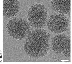
This electron micrograph documents the porous nature of the silica nanoparticles. These pores are large enough to allow entrance of a large number of NSA molecules. Here, they are protected until being taken up by the immune cells. At this point NSA is released and can stop the inflammatory processes.
