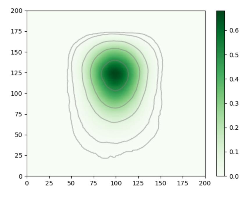
Section of a fuzzy pipe. The contour lines correspond to membership levels 0.001, 0.01, 0.1, 0.25, 0.5.
