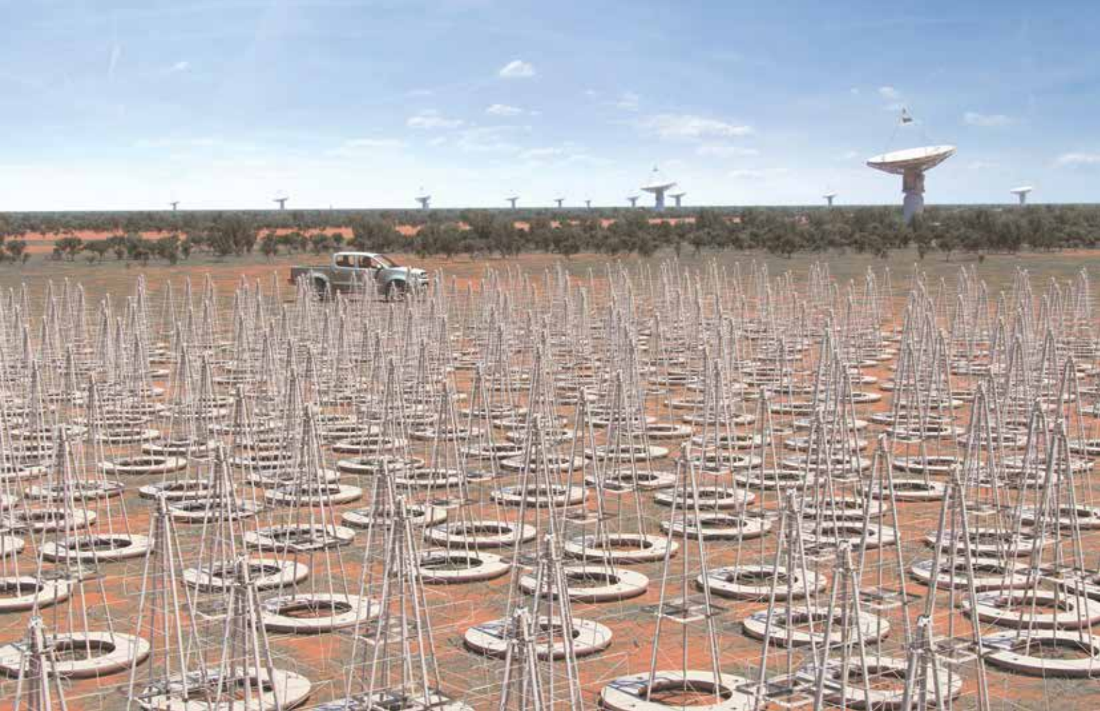
Figure 4 Close up artist rendition. Image of the Australian SKA LFAA (Low Frequency Aperture Array) instrument. These dipole antenna which will number in their hundreds of thousands will survey the radio sky in frequencies as low as 50Mhz. Credit: SKA Organisation/Swinburne Astronomy Productions
