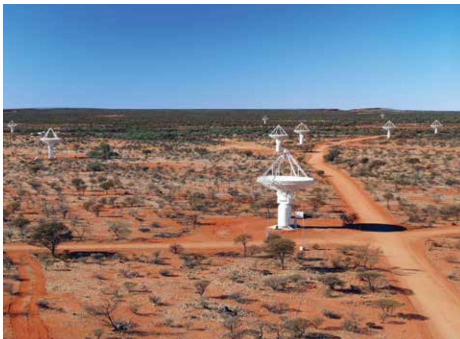
Figure 52 CSIRO's ASKAP antennas at the Murchison Radio-astronomy Observatory in Western Australia, installed with innovative phased array feed (PAF) receivers at the apex of the antenna. Credit: CSIRO.
