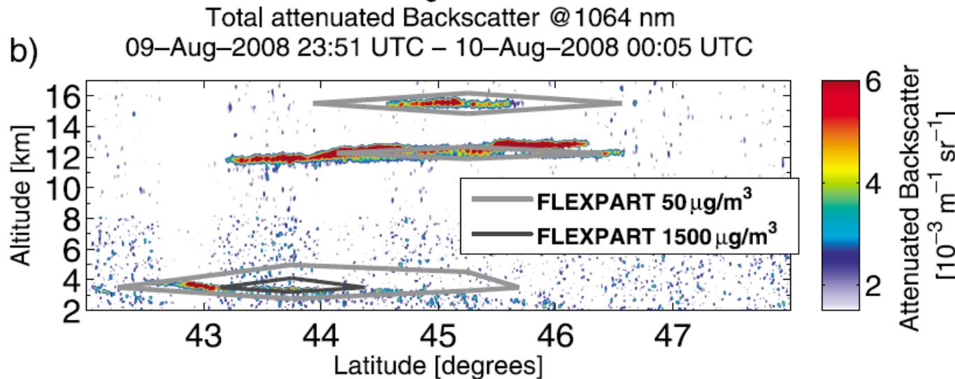
CALIOP: Lidar measurements along red line in (a)
