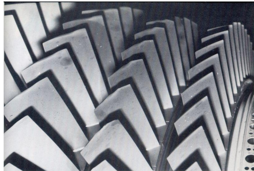
Effect of erosion on IP, 1, 2, 3 & 4 rotor blade.
