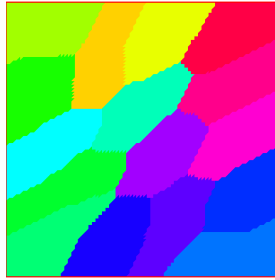
FIG. 7. On the left, number of iterations needed to reach convergence as the number of subdomains increases. On the right, example of decomposition into 16 subdomains using Metis.
